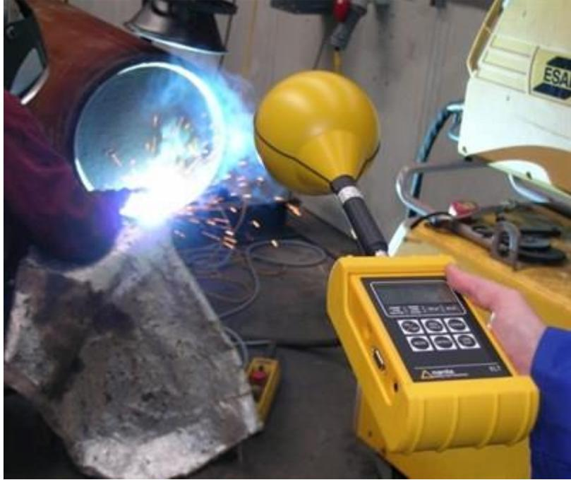
Figure 2. Equipment for measuring the magnetic field
