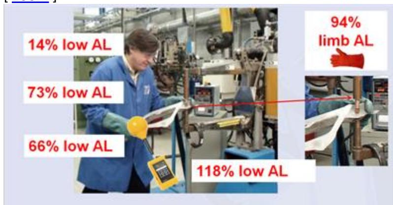
Figure 4 Assessment for resistance welding
