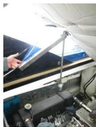
Suitable inline check valves local to each hydraulic cylinder should be installed to prevent the retraction of the hydraulic cylinders in the event of a loss of hydraulic pressure including hose failure. Suitable inline pressure relief device should also be fitted and appropriately set to prevent over pressurisation and/or pump overload.
